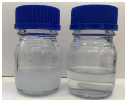
Figure 18. Demonstration of an unsuccessful (left) and successful (right) hydrolysis of the reagent.
