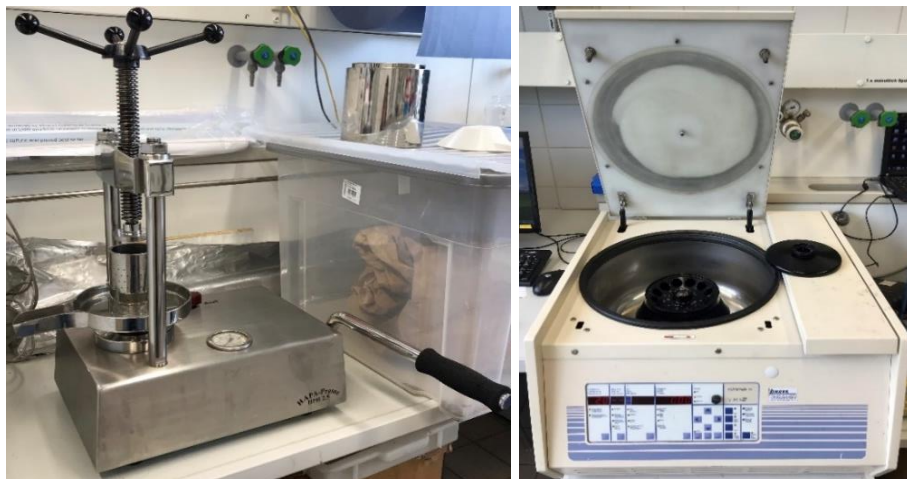
Figure 12. Representation of the press and centrifuge used in the extraction process.
